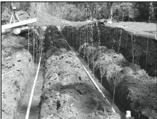
Figure 16. Measure squirt height
