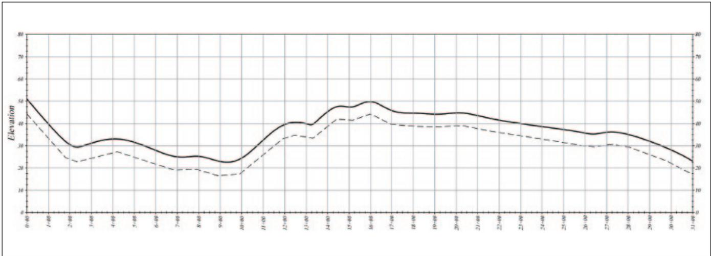
Figure 6. Typical pressure sewer profile, following the contour of the land.
