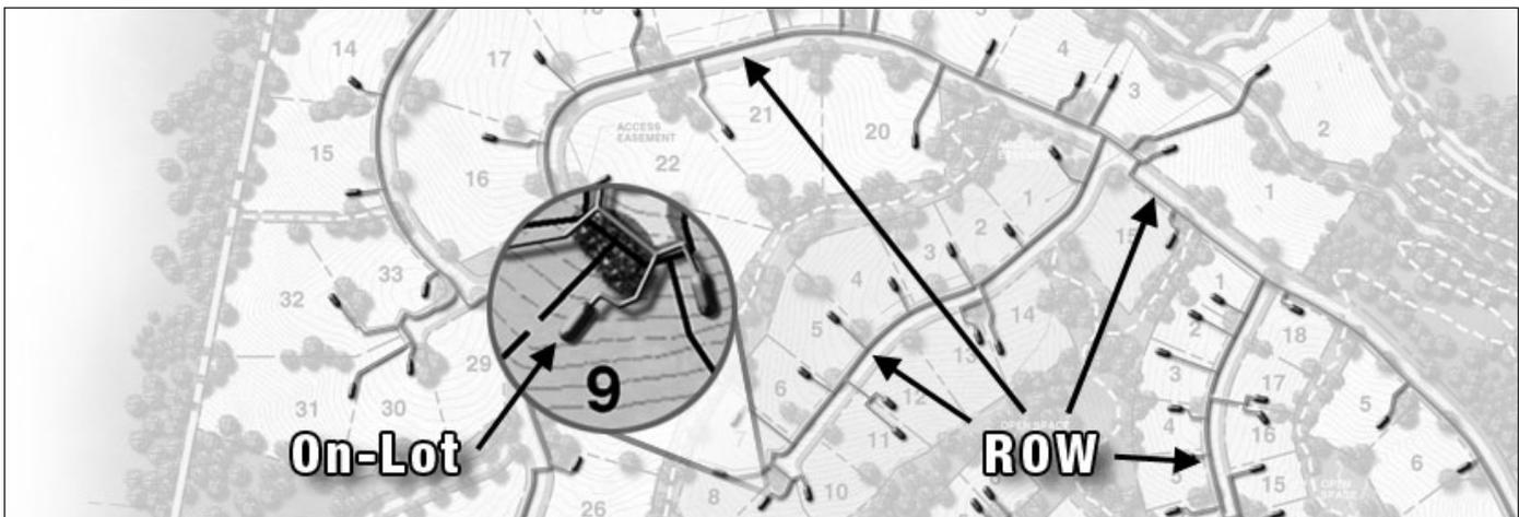
**Figure 1. Collection system costs include on-lot equipment and right-of-way components.**
