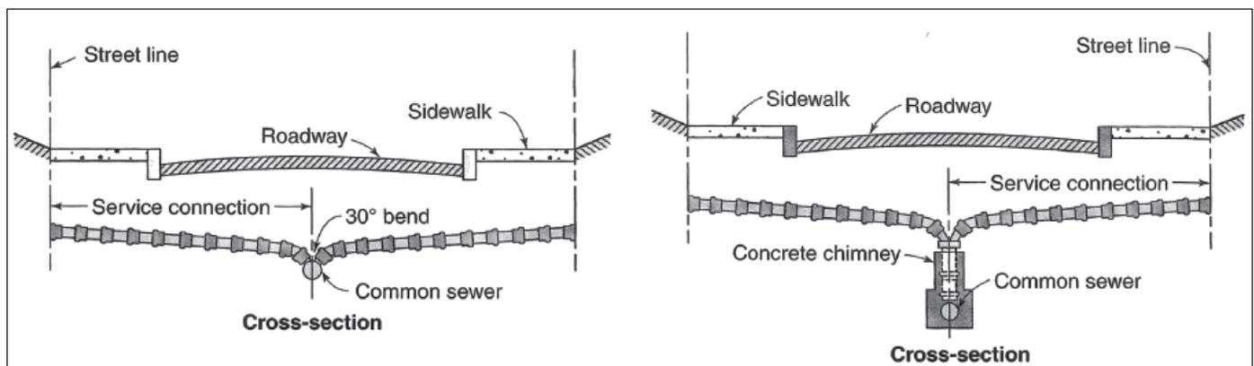
**Figure 5. Typical gravity sewer service lateral (Water Supply and Wastewater Removal, 2011).**
