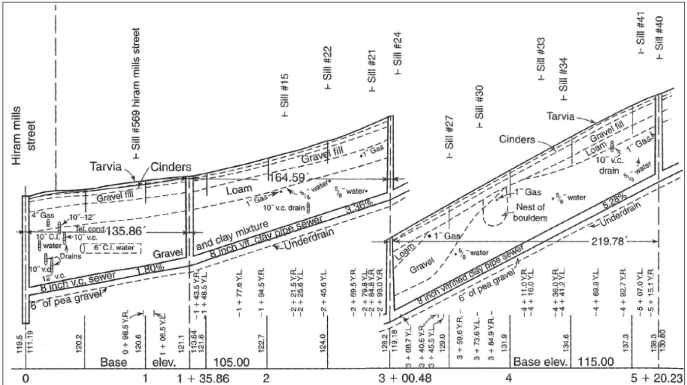
Figure 7. Profile of gravity sewer (*Water Supply and Wastewater Removal, 2011*).
