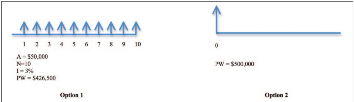
Figure 8. Economics of phasing in an Orenco Effluent Sewer system.
