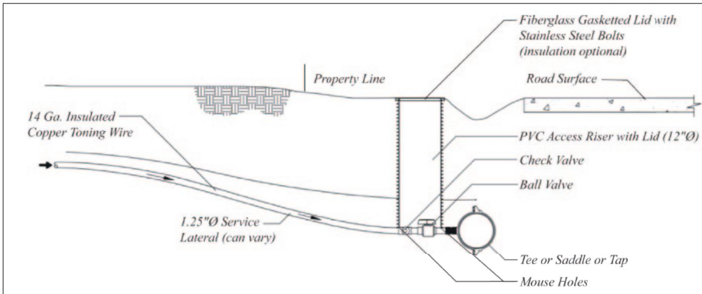
Figure 4. Pressure sewer service lateral.
